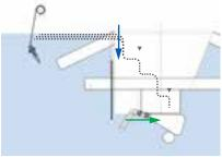
The release system can be adjusted according to the amount of the scum: height of opening gate before scraper approach, length of opening period.
