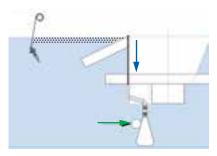
In the front part of the patented scum box is a scum gate that stops the water flow when the scraper flight is not at the scum hox.
